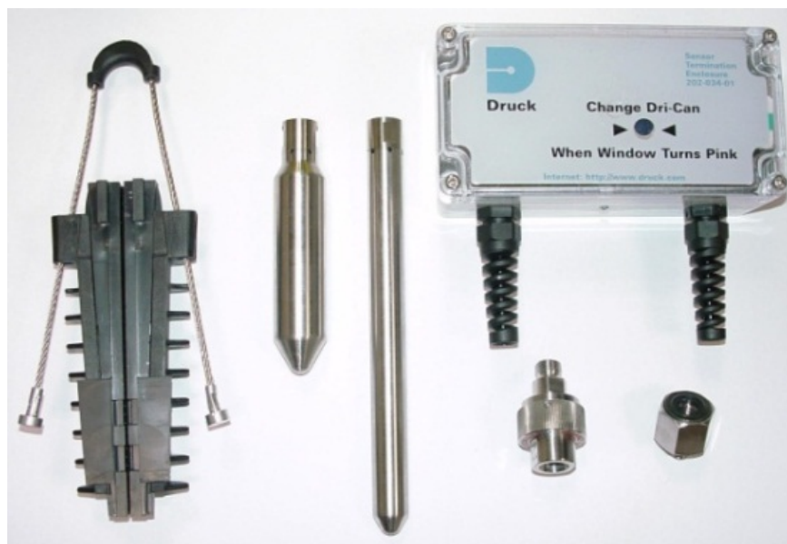
Figure 8.7: From left to right in picture are: Cable Clamp, Sink Weights, Sensor Termination Enclosure (STE Box), and below right are calibration adaptors.
